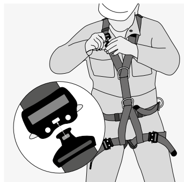
Repeat for right shoulder strap and connect the buckle. Ensure green spot can be seen in the receiver window
