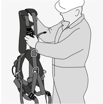
Hold harness by the shoulder straps and disconnect the chest fast release buckle
